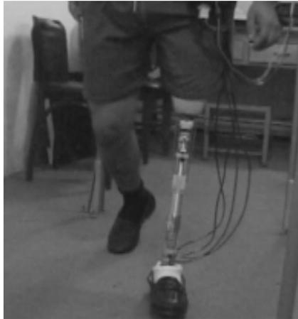
Figure 6. Transfemoral Prosthesis (Raptopoulos, 2003)
